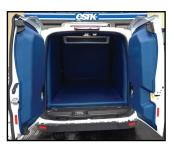
Our Transit fleet features 110 volt electric standby for easy stationary use. The vehicles are also wired for use of a 33 gallon ColdCube, so you can simultaneously store frozen and refrigerated goods in the same vehicle.
